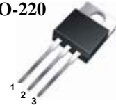
1. Gate 2. Drain 3. Source
